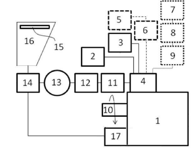
Fig. 3 Schematic diagram of the speed control system of wood chipper drive with a spark-ignition internal combustion engine; 1 - spark ignition engine, 2 - air filter, 3 - gasoline tank, 4 - carburetor, 5 - LPG gas tank, 6 - pressure reducer, 7 - CNG gas tank, 8 - high pressure reducer, 9 - low pressure reducer, 10 - output shaft, 11 - cen-trifugal mechanism, 12 - speed control lever, 13 - stepper motor, 14 - controller, 15 - sensors, 16 - supply channel, 17 - oil temperature sensor
