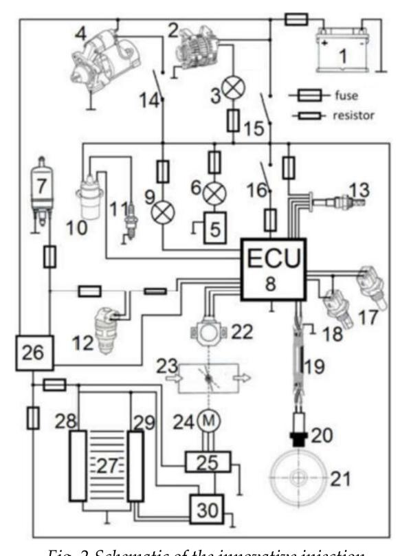
Fig. 2 Schematic of the innovative injection—ignition system
