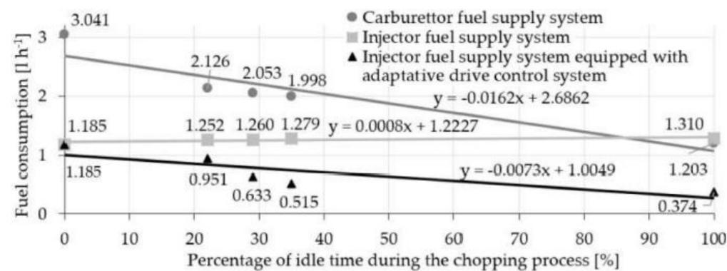
Fuel consumption under selected operating conditions: Transient exploitation conditions
