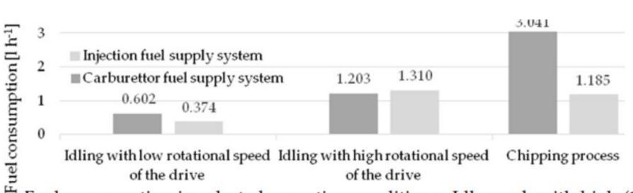
Fuel consumption in selected operating conditions: Idle work with high (1) and low (2) rotational speed, with a continuous chipping process (3).
