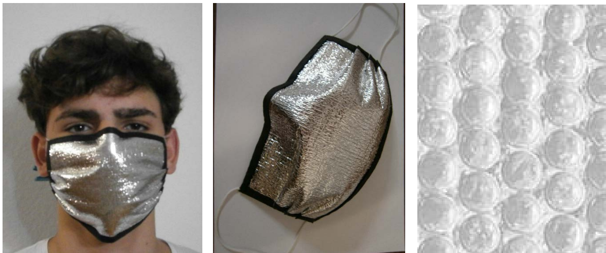
The mask with double-surface semi-spherical bubbles internal pad
