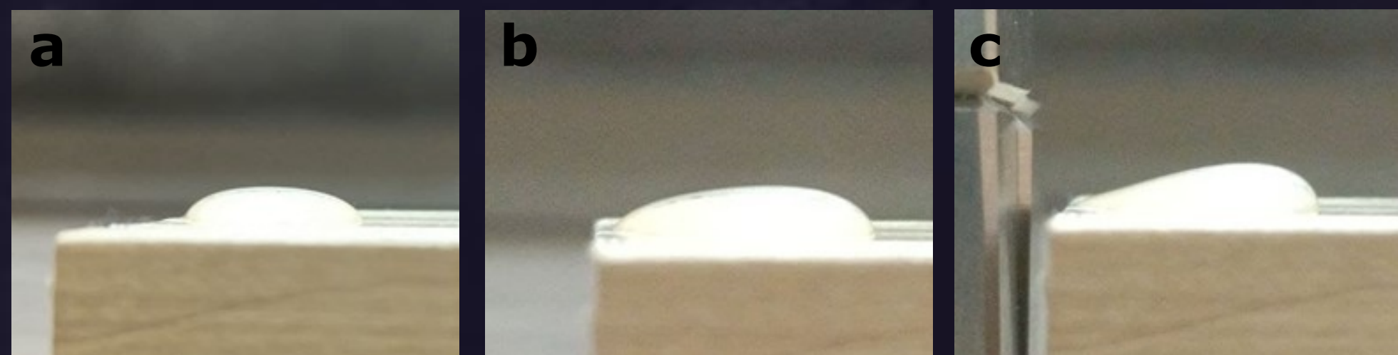
Fig. 3. Water without influence (a), under weak (b) and under strong influence of the magnetic field (c)
