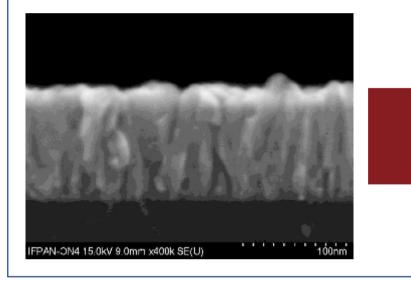
Precise thickness control (ZnO film)
