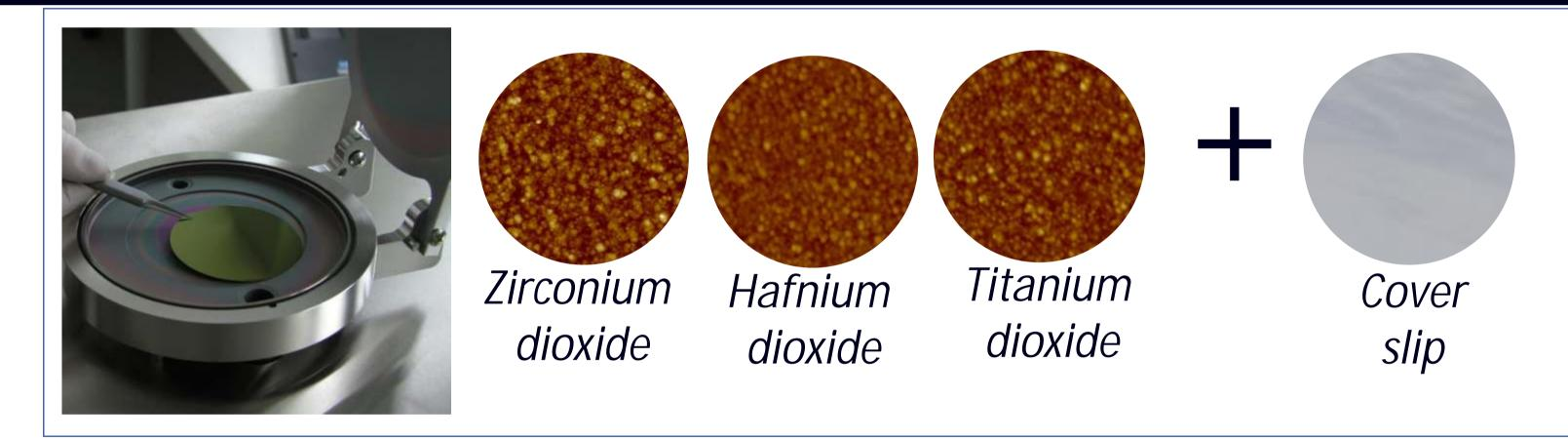
We test the oxides of transition metals for their biocompatibility with osteo-cells. We have investigated zirkonium dioxide, hafnium dioxide and titanium dioxide obtained by ALD technology. We studied the development of bone marrow stromal cells in contact with the ALD layers and observed different behaviour of such cells in relation to different oxides.
