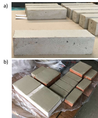
Fig. 1 Specimens a) rectangular 40x40x160mm b) on substrates made of masonry elements
