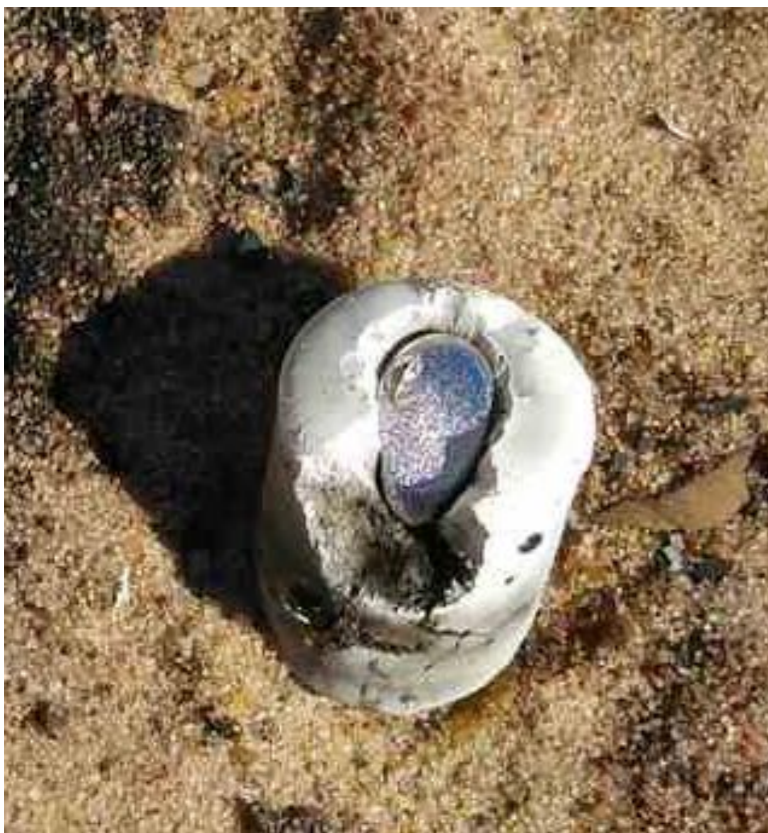
Forma tracona z gipsu zalana aluminium
