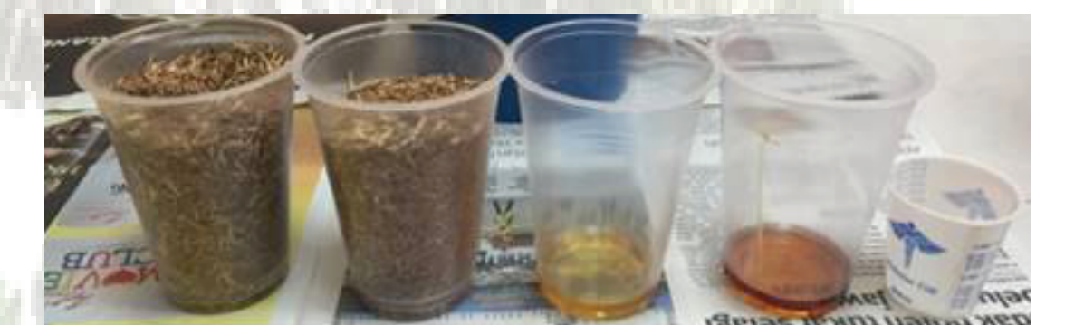
Preparation of Acacia waste particle & Palm Oil based Polyurethane Adhesive
