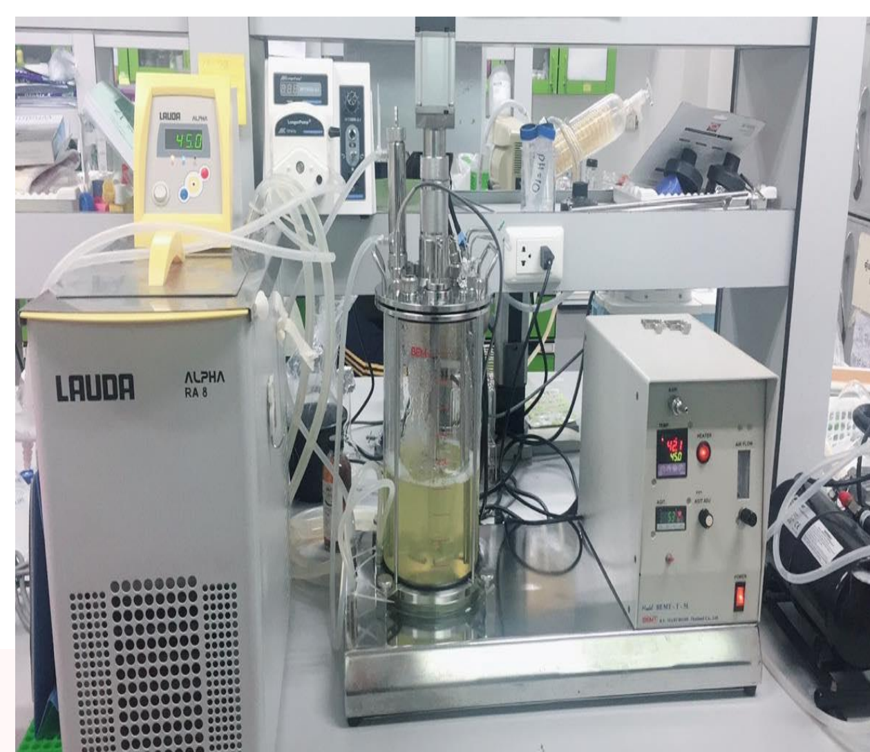
Enzymatic Hydrolysis in Stirred Tank Bioreactor
