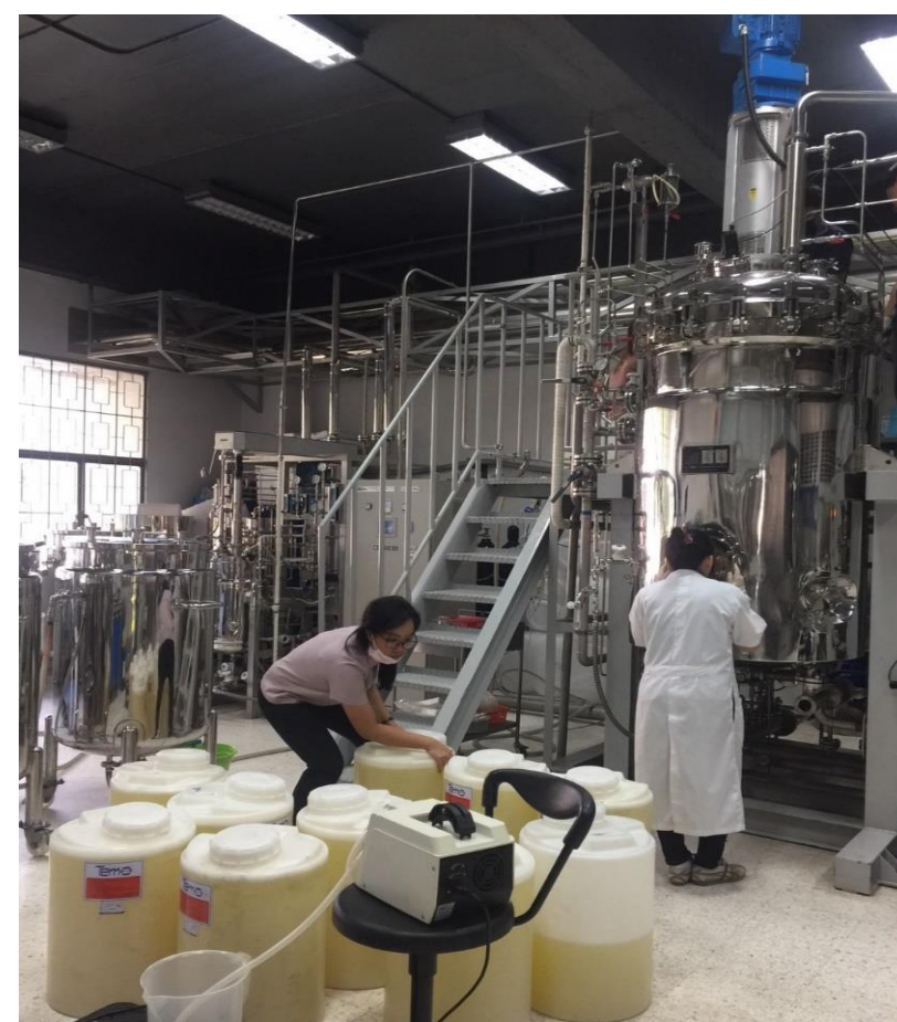
Hydrolysis in Pilot Scale Bioreactor
