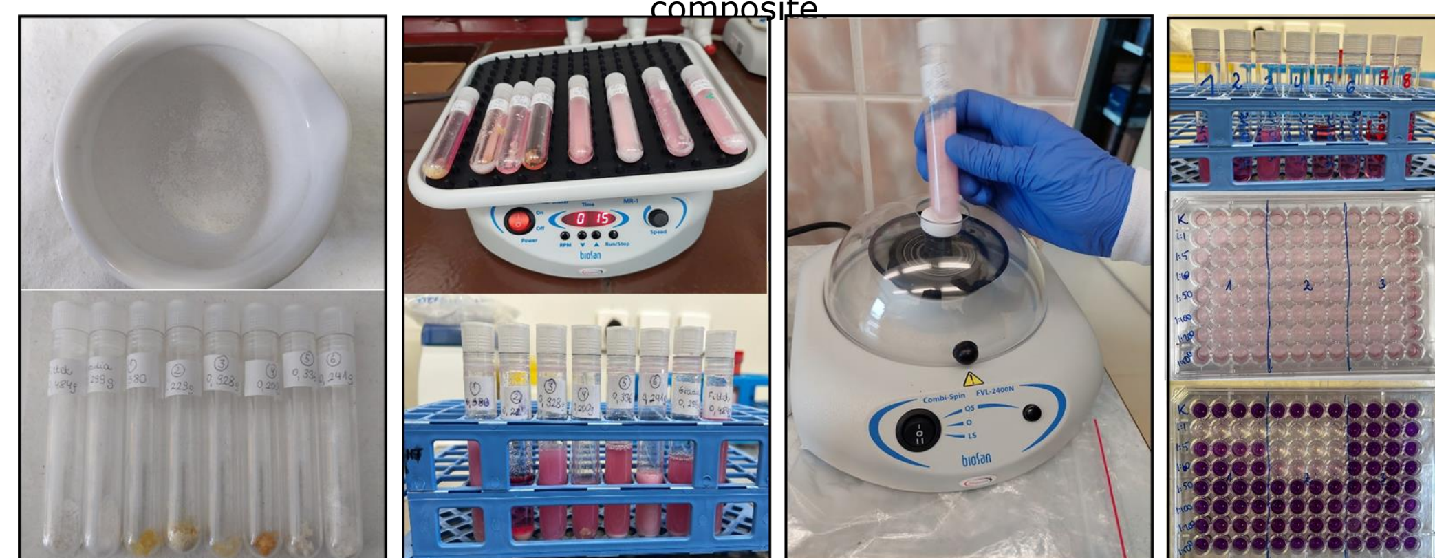
Fig. 6. Photographs demonstrating steps in the preparation of composites for cytotoxicity testing.
